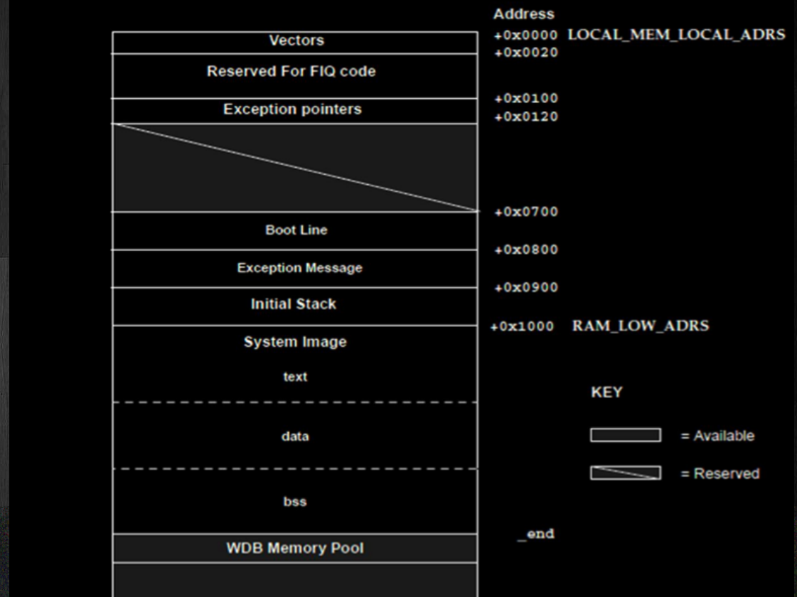
Figure G-2 VxWorks System Memory Layout (ARM)
